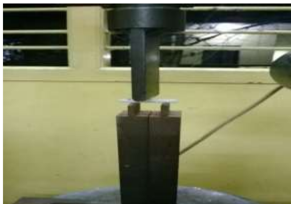
Fig -2 Photograph of Inter-laminar shear test (ILSS) specimen mounted on UTM.
