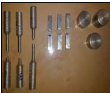
Figure (2): Experimented samples of Al8011-SiC composites.
