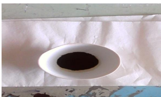
Figure-2: Nano powder ready for sintering
