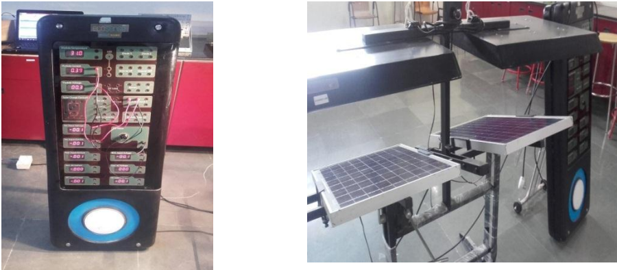
Figure 1: The Control Panel (left) and the PV modules I and II (right) used for this investigation
