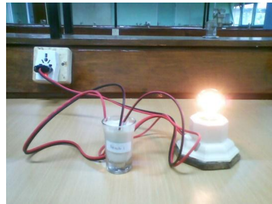
Fig. 3 Emulsion type test with electrical conductivity method
