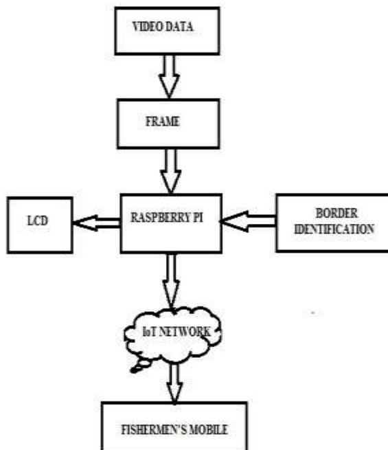
**Fig: 1 Block Representation of Smart aquatic fish monitoring**
