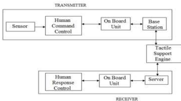
**Figure 2 Hardware Setup for Transmitter Vehicle and Receiver Vehicle**
