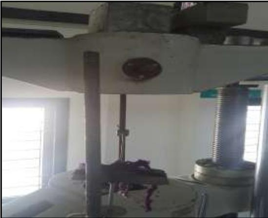
Figure 3. Testing of pull out specimens
