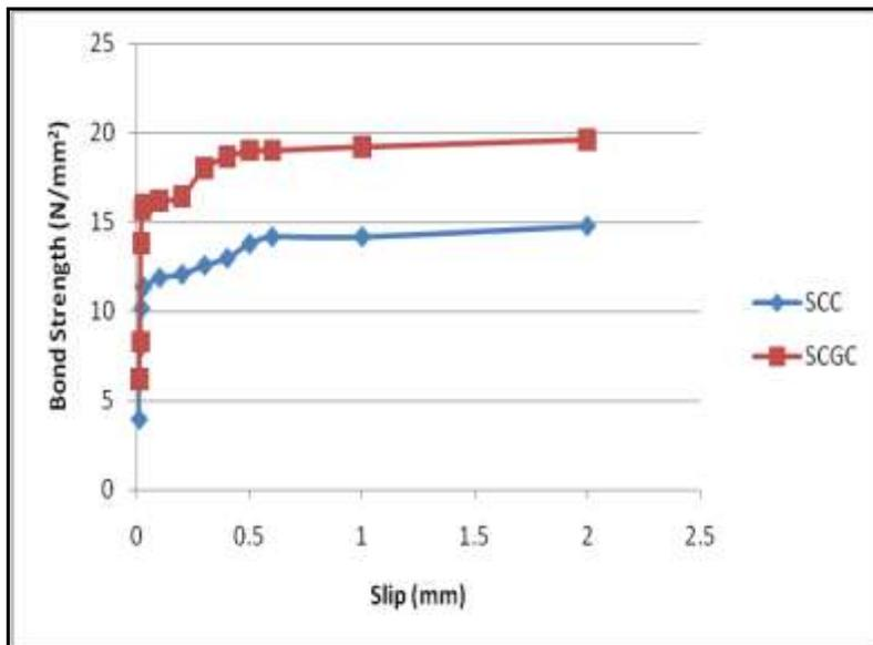
Figure 5. Bond Stress Vs. Slip of 12 mm Dia specimens
