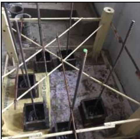
**Figure 2. Casting arrangement of pull out specimens**
