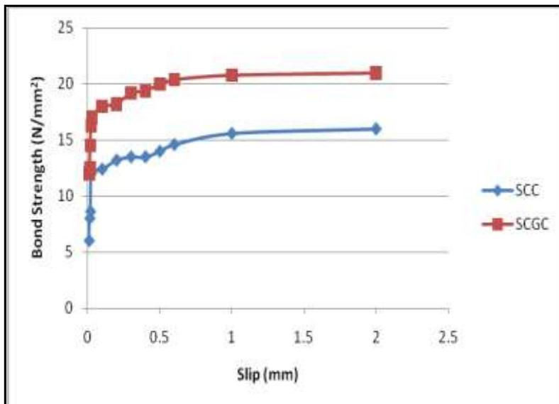
Figure 6. Bond Stress Vs. Slip variation of 16 mm Dia. Bar specimens
