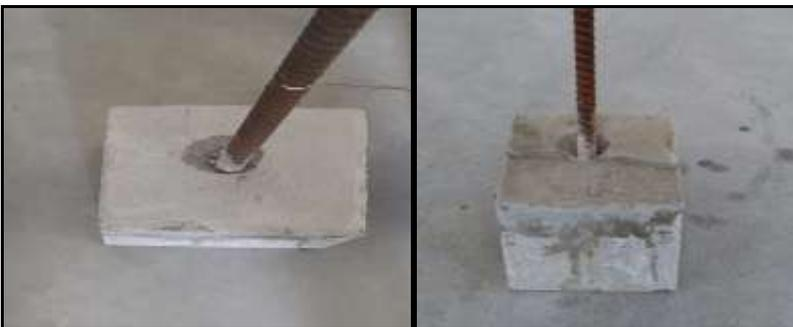
Figure 4. Failure of specimens in shear due to pull out of bars
