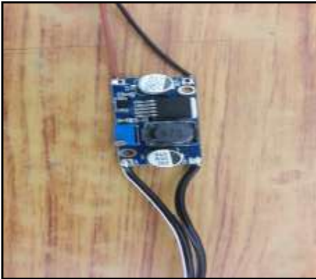
Figure 13: DC-DC Converter (Boost)
