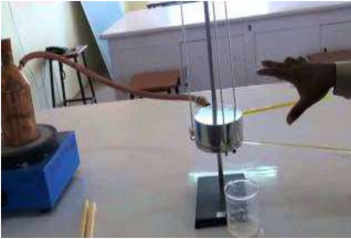
Figure 5. Configuration of Lee test of bad conductors and the temperature gradient through the sample
