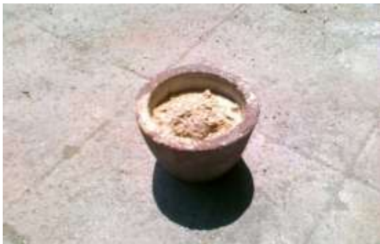
Figure 3.3.1 Pre heated Fly ash particles
