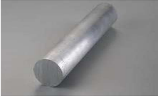
Figure 2.1 Aluminium alloy Al6061 80mm rod
