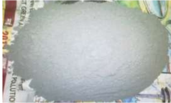
Figure 2.2 Fly ash of 50µm
