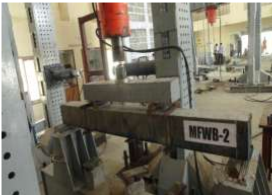
Fig 8. Fully wrapped beam with mechanical clamp
