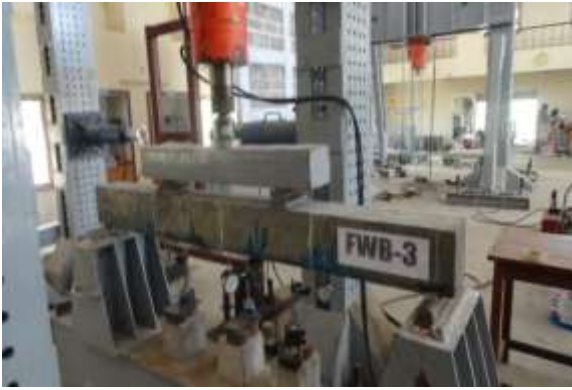
Fig 6. CFRP fully wrapped on its tension zone of precracked beam
