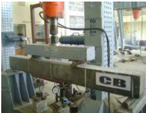
Fig 4. Testing of control beam (concrete with glass fibre without wrapping)
