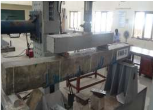
Fig 7. Cracks formation on CFRP wrapped concrete beam
