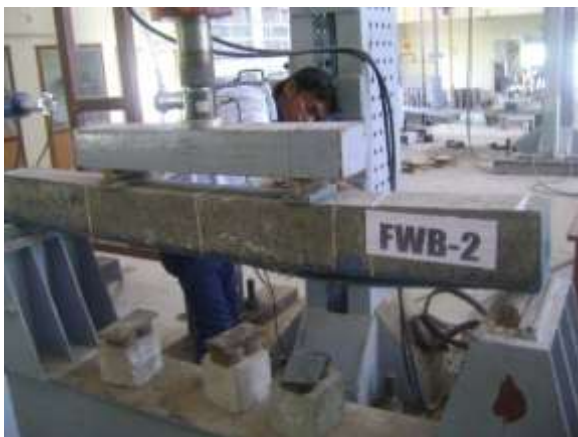
Fig 8. Crack patterns observed in fully wrapping beam
