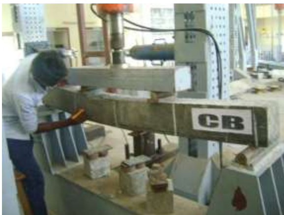
Fig4. Deflection and Crack patterns observed in control beam under loading
