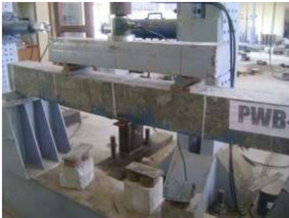
Fig 6. Crack patterns observed in partially wrapping beam
