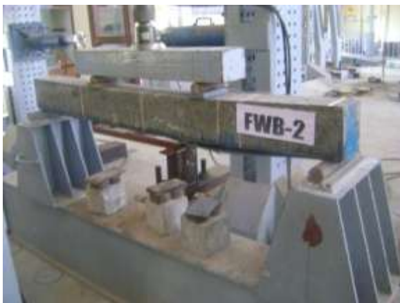
Fig 7. CFRP fully wrapped on its tension zone
