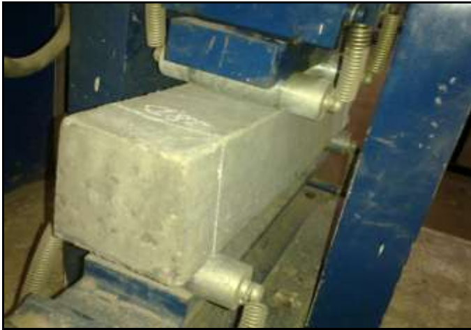
Fig3: Flexural strength testing on prism
