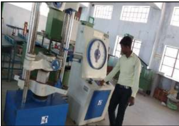
Fig1: Compressive strength test on cube
