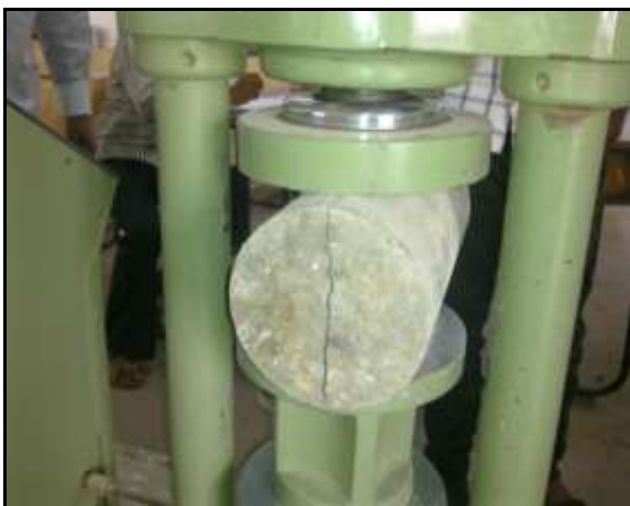
Fig2. Split Tensile strength test on cylinder
