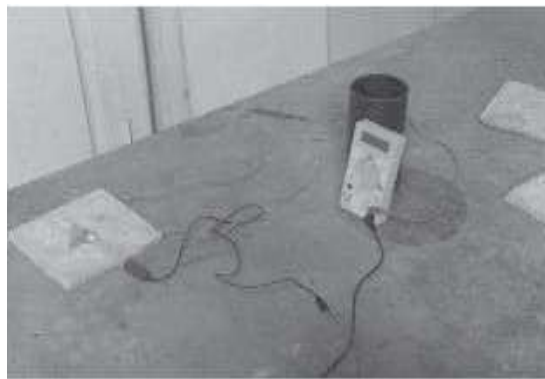
Fig8. Electrochemical Potential Measurement using Saturated Calomel reference Electrode and Multimeter
