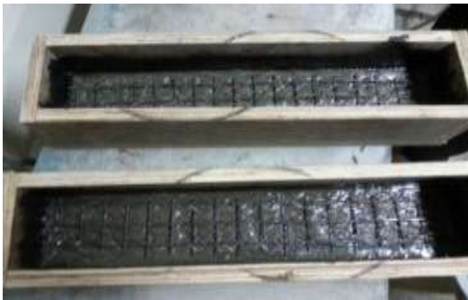
Fig 1. Casting of ferrocement and ferro-geopolymer mortar beams
