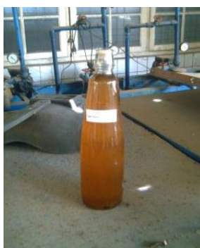
Figure 1. Cinnamon liquid smoke on pyrolysis temperature of 400°C
