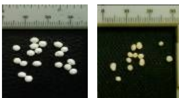
Fig. 1. Floating-mucoadhesive alginate beads containing Al(OH) 3 and Mg(OH) 2 (F3). (a) Beads of F3 for in vitro evaluation; (b) Beads of F3 for in vivo evaluation.
