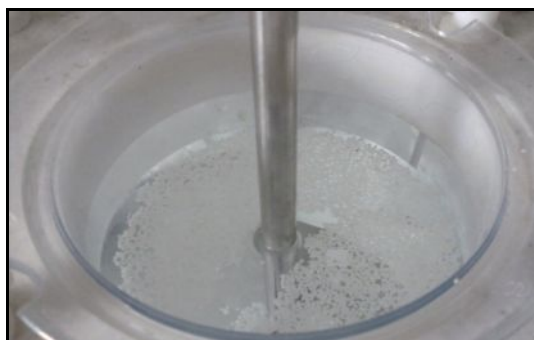
Figure 2: In vitro buoyancy study of Cimetidine floating microspheres
