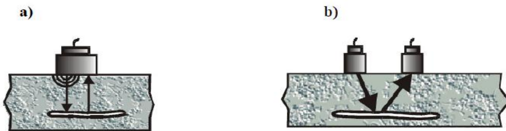
Figure 2: The ultrasonic echo method of concrete: a- receiving and transmitting transducer, b- double transducer
