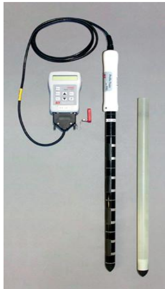
Fig. 2: Profile probe for measuring soil moisture content
