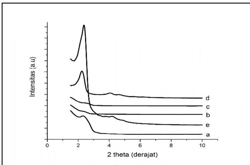
**Figure 1. X-ray diffraction pattern of the MCM-41 synthesized under sonication time variations: (a) 30, (b) 60, (c) 90, (d) 120, and (e) 150 min.**
