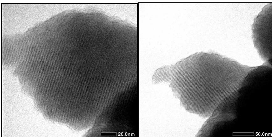
**Figure 3. The TEM image of MCM-41 sonicated for 150 min. with the scale of 20 nm and 50 nm**
