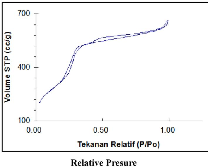
**Figure 2. Adsorption-desorption isotherm of N<sub>2</sub> for MCM-41 sonicated for 150 min**
