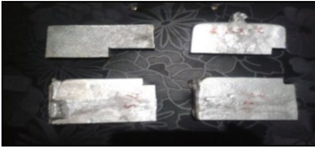
Fig.1:Prepared specimen, clockwise Al6061, Al-NCG 2.5%, Al-NCG 10%,Al-NCG 5%.
