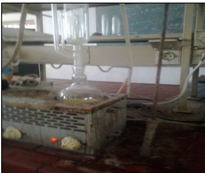
Figure 3. Soxhlet extractor setup for oil extraction
