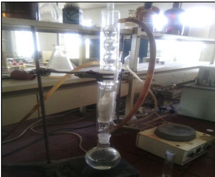
Figure 4: Soxhlet apparatus setup used for the oil extraction
