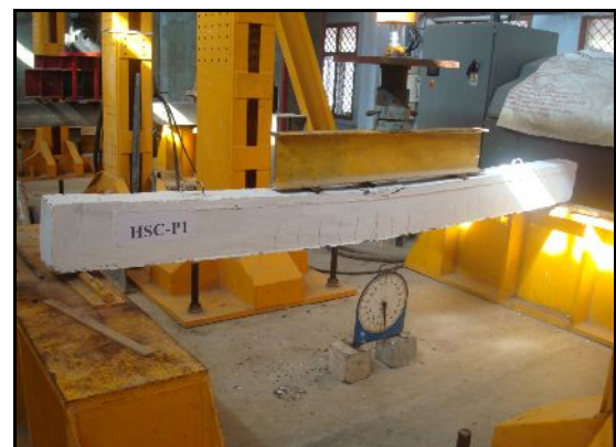
Fig. 3. View of Cyclic Load Test of Beam
