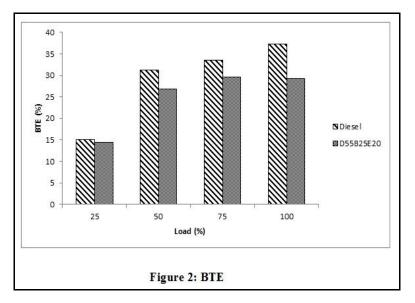
The Figure 2 shows the variation of Brake thermal efficiency of the blend as compared to diesel with respect to load. It is observed that the BTE of D55B25E20 is lower than that of diesel due to lower calorific value of the blend as compared to diesel.
