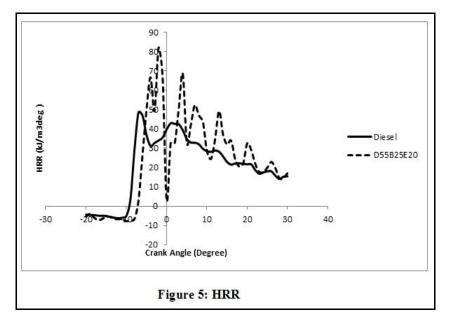
The Figure 5 shows the variation of heat release rate of blends at full load as compared to diesel with respect to Crank angle. The maximum heat release for diesel was 47 kJ/m3deg at 6°CA, and for D55B25E20 was 82 kJ/m3deg at -2°CA. It is observed that the maximum heat release of the blends is higher than that of diesel. This can be due to higher oxygen content of the fuel. Also, the reactivity of the oxygen is better at higher temperatures.
