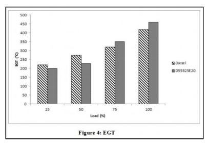
The Figure 4 shows the variation of Exhaust Gas temperature of D55B25E20 as compared to diesel with respect to load. It is observed that the EGT of the blend is lower than diesel up to part load. This is due to higher latent heat of evaporation of the fuel blend. Also, with the increase of load, the EGT of the blend is increasing.
