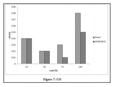
The Figure 7 shows the variation of Carbon Monoxide level of blends as compared to diesel with respect to load. It is observed that the CO of blend is lower than that of diesel after part load. At higher loads, the average temperature of the combustion chamber increases, thereby leading to more oxygen activity of the blend. Hence, better complete combustion of the fuel takes place, reducing CO emissions.
