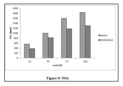
The Figure9 shows the variation of oxide of nitrogen level of the blend as compared to diesel with respect to load. It is observed that the  $NO_x$  of blendis lower than that of diesel. This is due to ethanol content which reduces the combustion temperature and prevents the formation of  $NO_x$ . Also, due to low calorific value of the blends, the cylinder temperature is lower than that of diesel. However, at full load, the  $NO_x$  emissions are higher as compared to lower loads.
