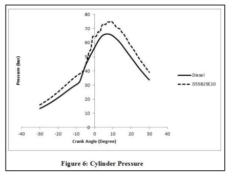
The Figure 6 shows the variation of pressure of blends at full load as compared to diesel with respect to Crank angle. The maximum pressure for diesel was 66 bar at 7°CA, and for D55B25E20 was 75 bar at 6°CA .It is observed that the cylinder pressure of both the blends is higher than that of diesel. This can be due to rapid combustion due to the accumulation of the fuel.
