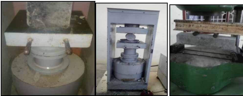
Figure 4. Test setup for Compressive, Spilt tension, Flexural strength
