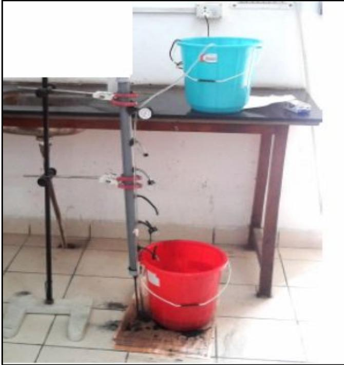
**Figure 2 Packed bed column in operation**
