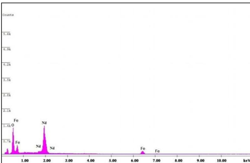
**Fig. 3 EDAX spectra for NdFeO<sub>3</sub> ceramics**
