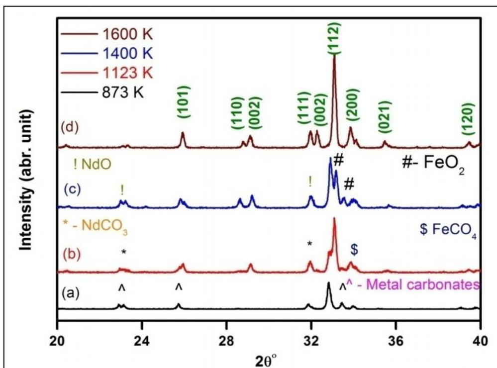
Fig. 1. Powder XRD for synthesized powder
