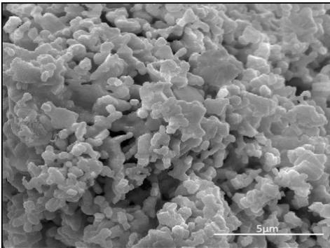
**Fig.2. HRSEM image of NdFeO<sub>3</sub> ceramics**
