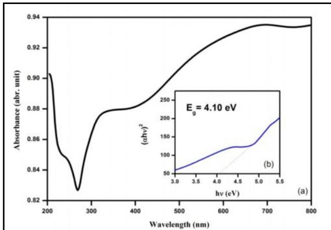
**Fig. 4 (a) Optical absorption spectrum of NdFeO<sub>3</sub> powder, and inset graph (b) Optical band gap.**
