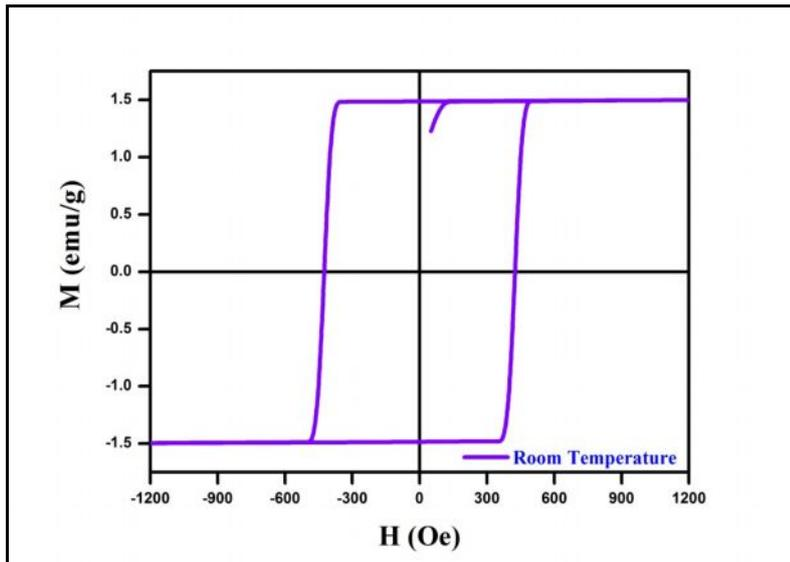
**Fig. 5 MH loop for NdFeO<sub>3</sub> ceramics.**
