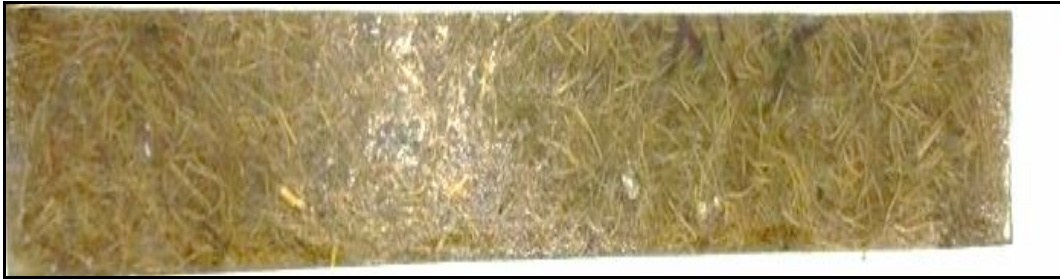
Figure 7: Cut section of coir reinforced composite plate
