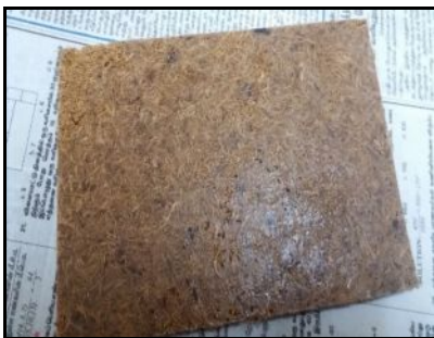
Figure 4: Composite plate of 30% coir and 70% epoxy resin
