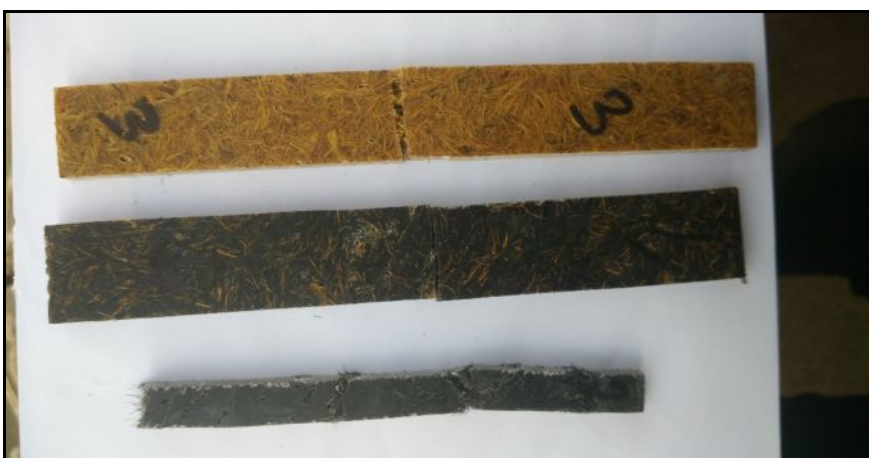
Figure 11: Tested samples for impact, tensile and flexural strengths.
