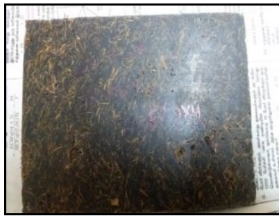
Figure 5: Composite plate of 10% coir and 10% hair with 80% epoxy resin
