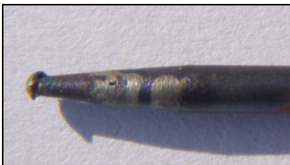
Fig. 2 Conical tip profile of 1.6mm electrode diameter.
