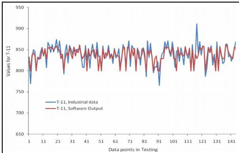
**Fig. A.2 Values of T-11 obtained from industry and predicted from software**
