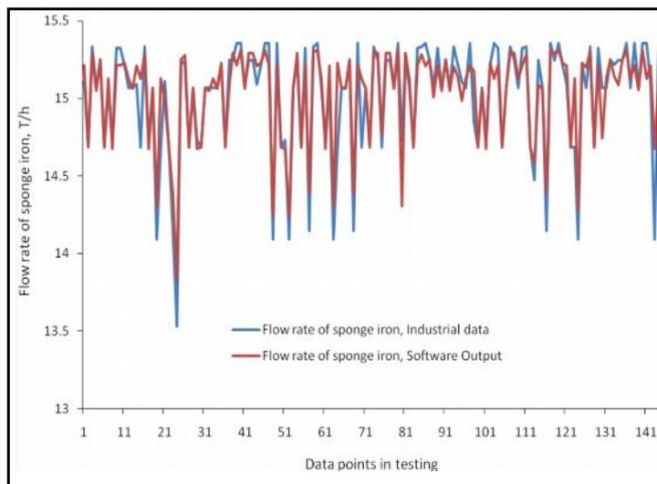
**Fig. 5** Flow rate of sponge iron obtained from industry and predicted from software
