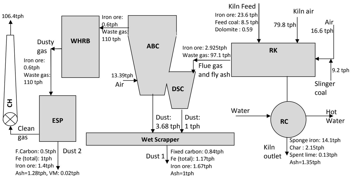
Fig. 1. Process flow diagram of sponge iron process
