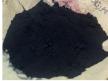
Fig.12: Crumb rubber used in the concrete mix
