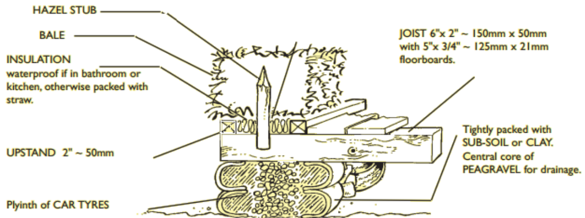
Fig.9: section through tires-parallel to joints (Amazon nails, 18 )
