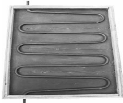
Figure 1. Absorber of a flat plate solar collector with a galvanized pipes and galvanized sheet 29
