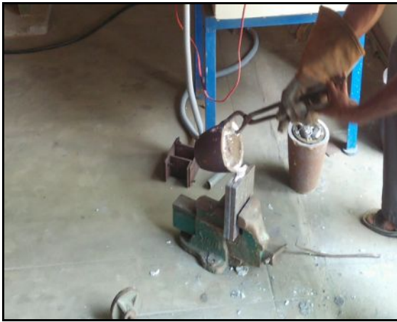
Figure.3. Pouring metal into the mould cavity
