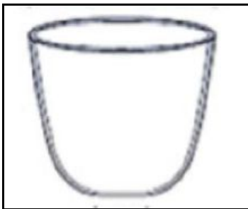
Figure 2.4 shows the graphite crucible for melting the Aluminium bar and TiB_2 .
