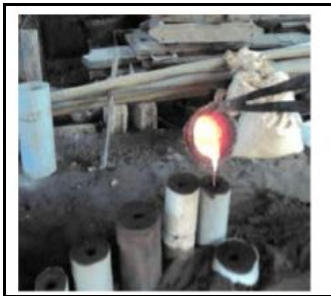
Figure 2.3 shows while pouring molten metal into the sand.
