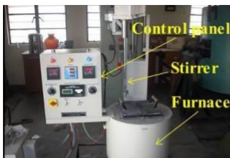
Figure 2.1 shows the experimental set up of stir casting method.
