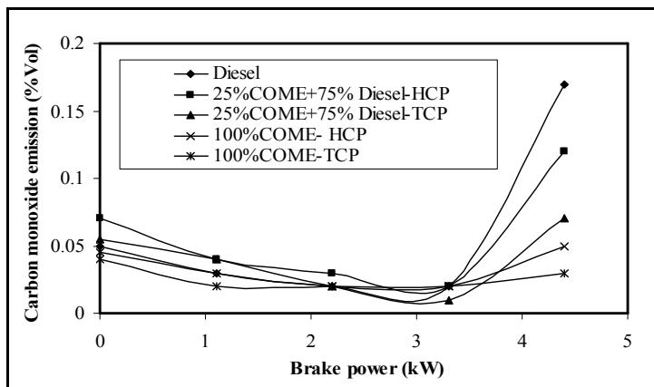
**Fig.6 Carbon monoxide emission Vs BP**
