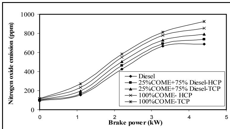
**Fig. 8 Nitrogen oxide emission Vs BP**
