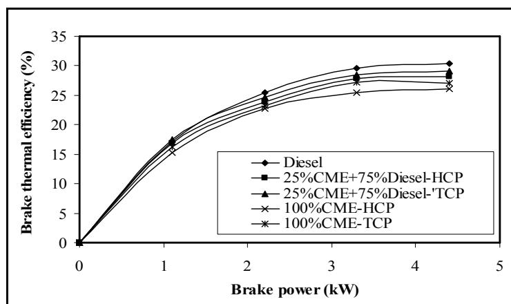
**Fig.3 Brake thermal efficiency Vs BP**
