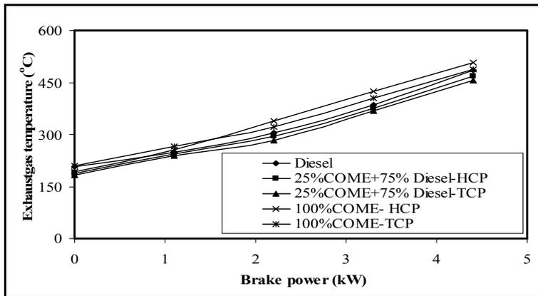
**Fig.5 Exhaust gas temperature Vs BP**
