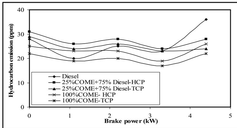
**Fig.7 Hydrocarbon emission Vs BP**
