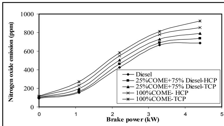
**Fig. 8 Nitrogen oxide emission Vs BP**
