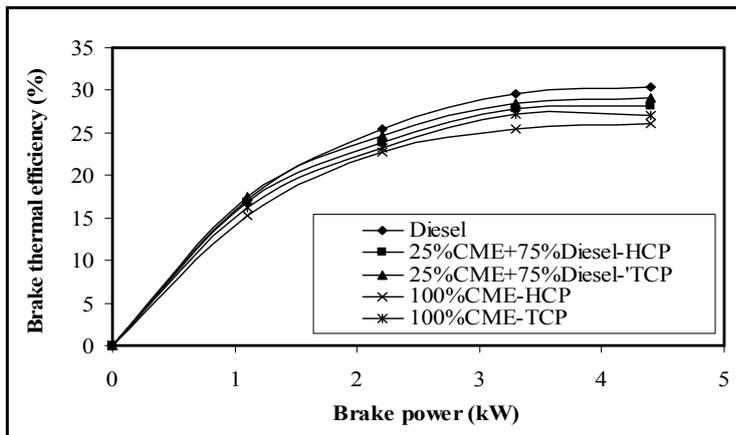
Fig.3 Brake thermal efficiency Vs BP
