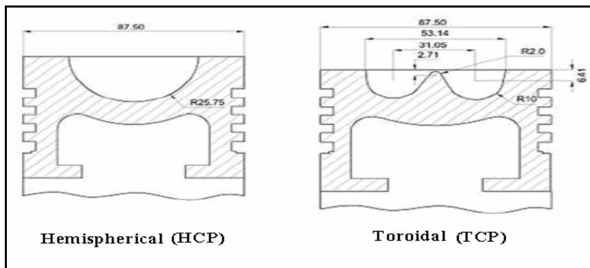
**Fig. 2 Modification of Piston bowl (all dimensions in mm)**
