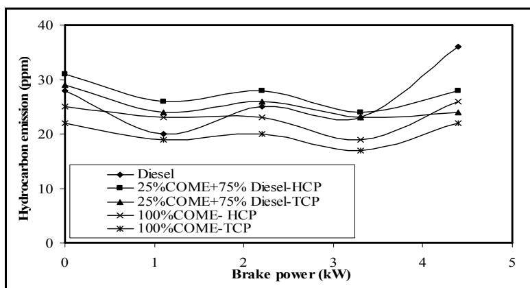
**Fig.7 Hydrocarbon emission Vs BP**
