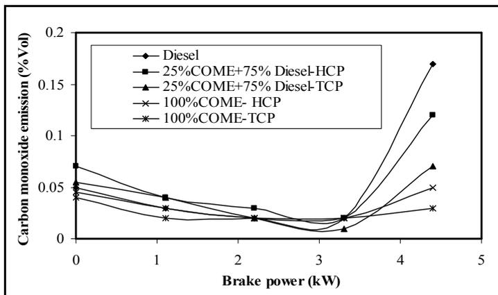
**Fig.6 Carbon monoxide emission Vs BP**
