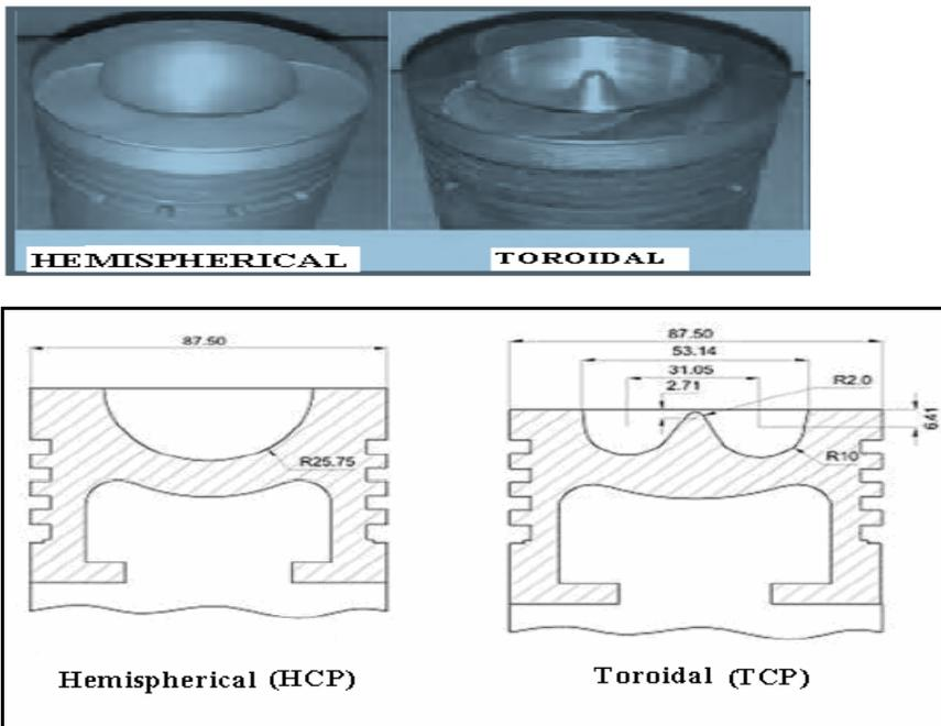
Fig. 2 Modification of Piston bowl (all dimensions in mm)
