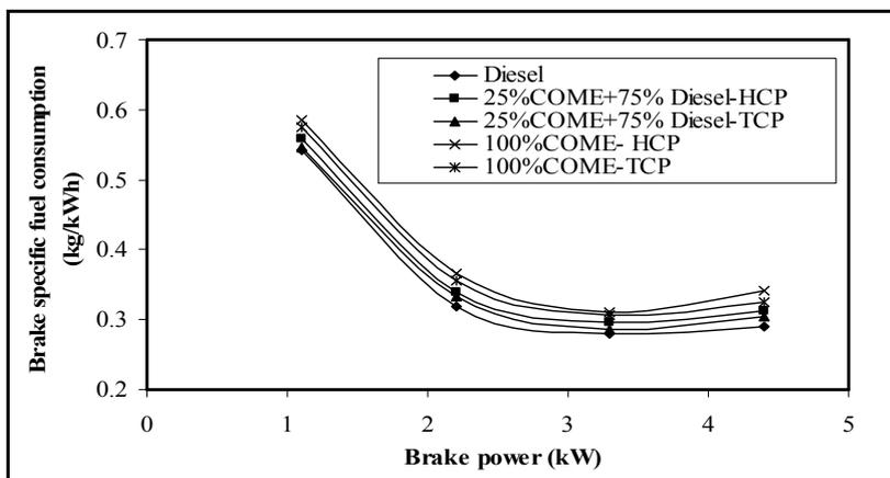
Fig.4 Brake specific fuel consumption Vs BP
