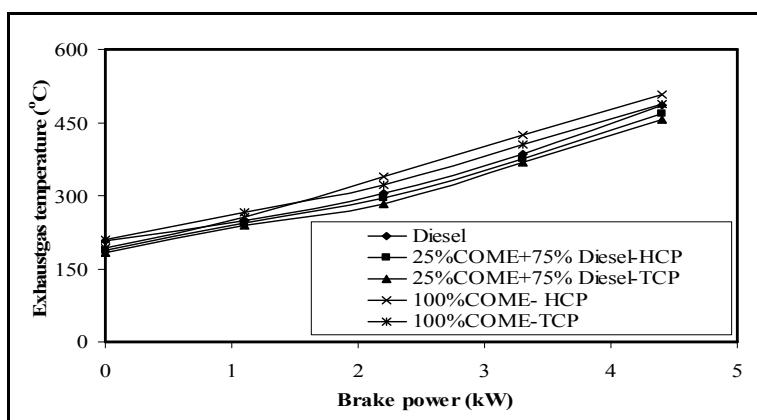
**Fig.5 Exhaust gas temperature Vs BP**
