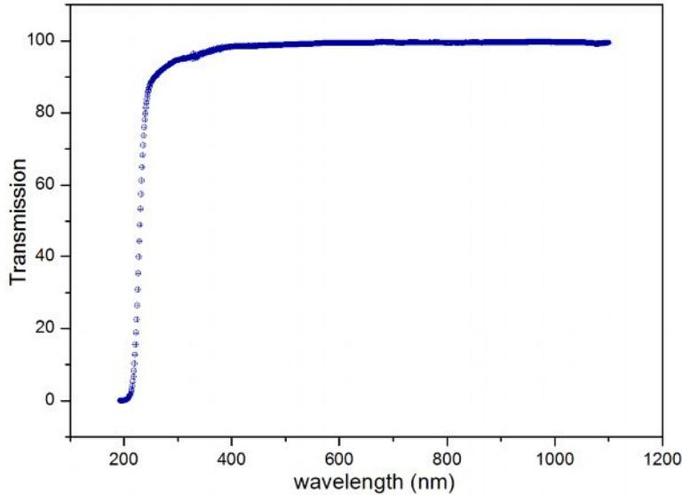
Fig. 3.3. UV-Visible Spectrum of LPS crystals
