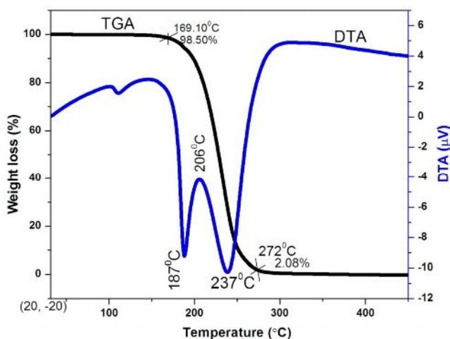
Fig. 3.4. TGA and DTA curve of LPS crystals
