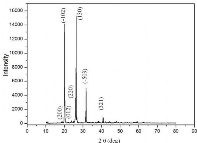
**Fig. 3.1. Powder X-Ray Diffraction pattern of LPS crystals**
