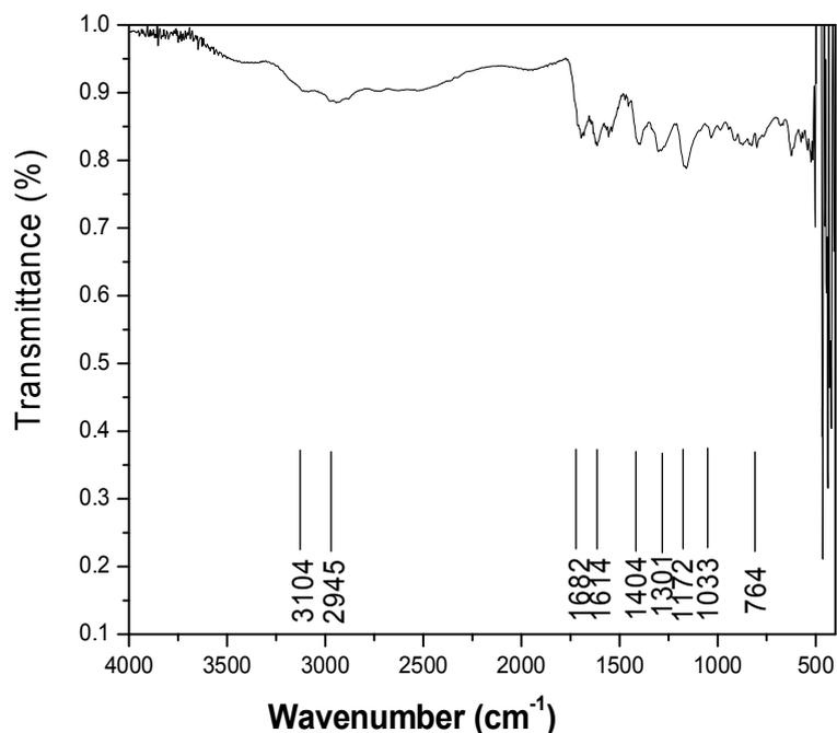
**Fig. 3.2. FTIR spectrum of LPS crystals**
