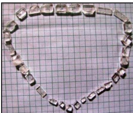
**Fig.1: L-Th Doped Seed Crystals**
