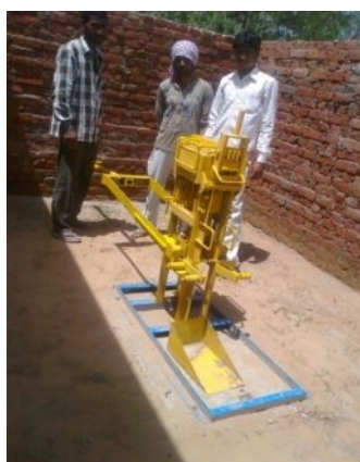
Fig. 3 Photograph of the installed Balaram Mud Block Machine
