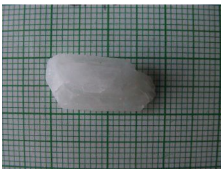
Fig. 2 Photograph of GGLY Crystal grown from Guanidine hydrochloride
