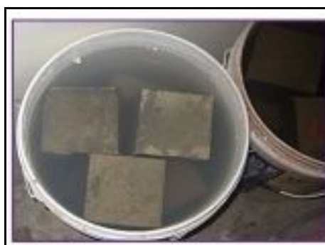
Fig.2 Cubes in curing
