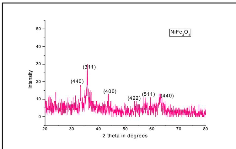
**Fig.1. XRD pattern of the NiFe<sub>2</sub>O<sub>4</sub> nanoparticles**
