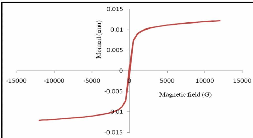
**Fig. 3 Magnetic hysteresis loop of Nickel ferrite Nanoparticles**
