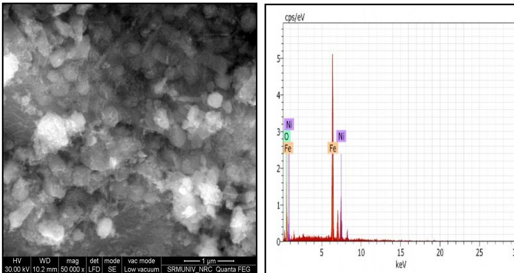
**Fig.2 SEM and EDX images of NiFe<sub>2</sub>O<sub>4</sub> NPs**
