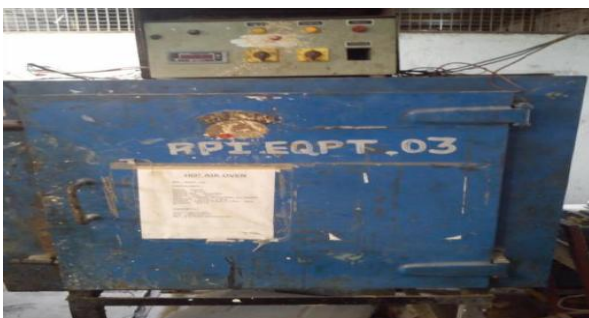
Figure 3. Hot Air Oven
