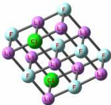
Figure.1 (b) Structure of Cl substituted cubic LiF nanostructure
