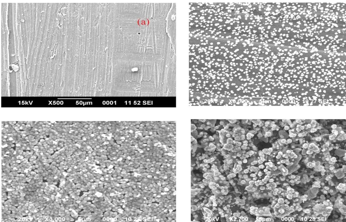
**Fig.2. SEM pictures of NiFeCr films electrodeposited from sulphate bath at (a)0.5A/dm<sup>2</sup> (b)1A/ dm<sup>2</sup> (c) 1.5 A/ dm<sup>2</sup>(d) 2A/ dm<sup>2</sup>**
