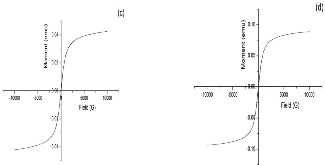
**Fig.3. VSM graphs of NiFeCr films electrodeposited from sulphate bath at (a)0.5A/dm<sup>2</sup> (b)1A/ dm<sup>2</sup> (c) 1.5 A/ dm<sup>2</sup>(d) 2A/ dm<sup>2</sup>**
