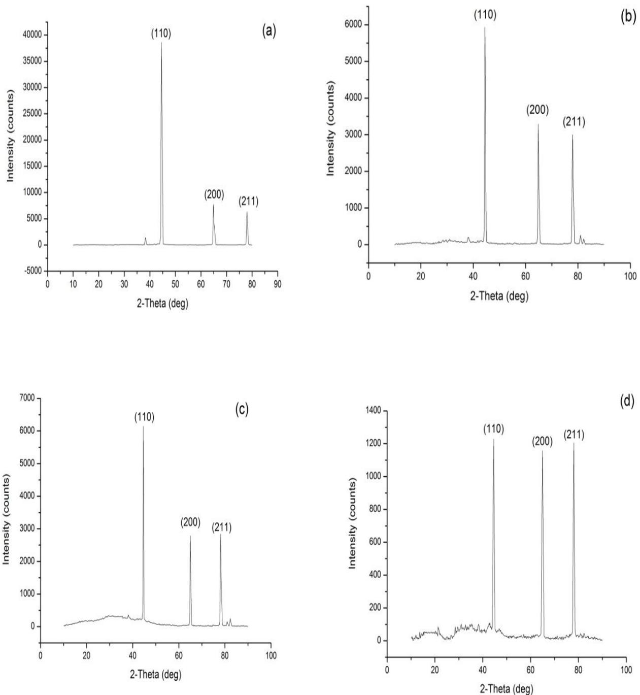
**Fig.3. XRD patterns of NiFeCr films electrodeposited from sulphate bath at (a)0.5A/dm<sup>2</sup> (b)1A/ dm<sup>2</sup> (c) 1.5 A/ dm<sup>2</sup>(d) 2A/ dm<sup>2</sup>**
