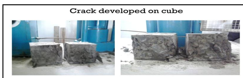
Fig-4: Different crack Patterns
