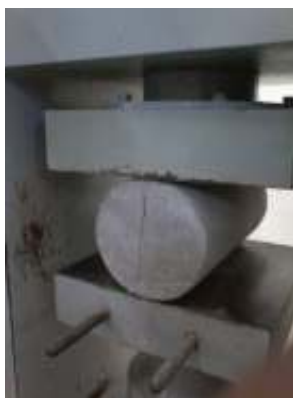
Fig.4. Test setup for split tensile strength
