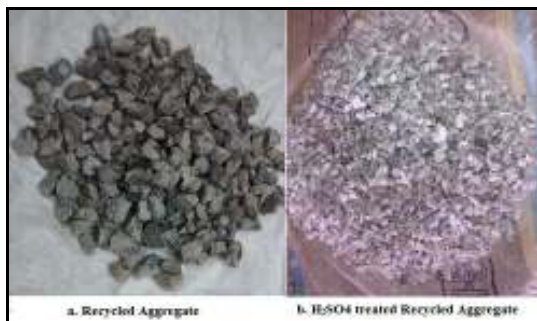
Fig.1 Recycled aggregates before and after treatment
