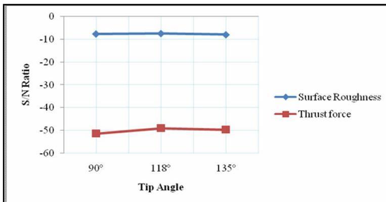
**Figure 4 Effect of cutting point angle on the responses**
